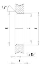
Installation direction: o-ring sits on chamfer.
